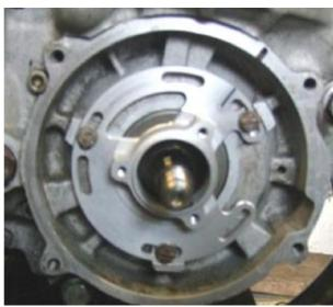
Unfasten the 3 screws M4x25, which hold the stator on its base but do not opull the wire completely trough the plate to avoid setting the stator back in the wrong position.
