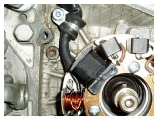
In KTM engines secure the cable with the stock cable holder or some small pipe clamp as shown here.
