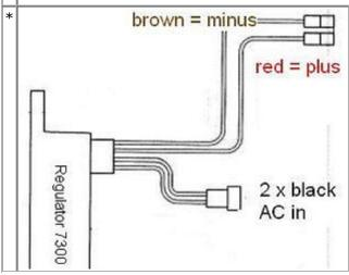
The new regulator/rectifier has 4 wires
