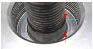
Further, you must check the end of the crank taper against the bottom surface of the puller hole of the rotor. With some engines the taper may be slightly above the bottom of the opening which will prevent the nut fastening the rotor securely if not detected and cured by adding a shim or in bad cases a distance piece. The rotor would slip in that case, making timing unsuitable.
